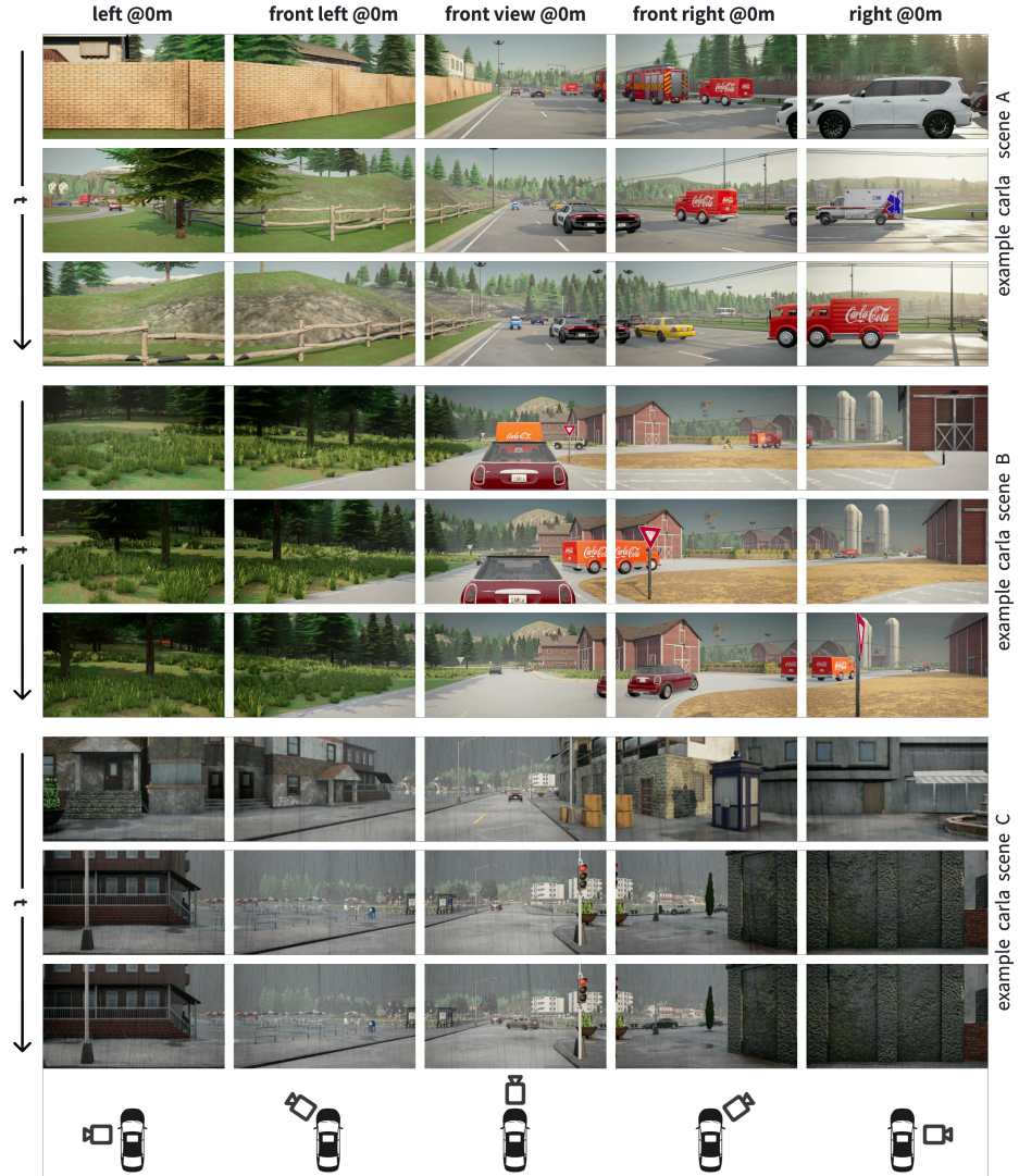
Fig.15: Multi-view camera observations in the Para4D dataset. Para4D simultaneously captures synchronized images from five ego-vehicle camera views for each parallel trajectory, following the same camera configuration as the Waymo dataset. Each row shows consecutive temporal frames from different driving scenes. This multi-view and temporally consistent setup is designed to support the training and evaluation of NVS methods.
