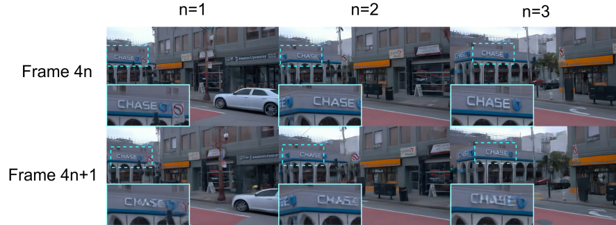
Fig. 18: Visualization of the temporal inconsistency caused by WanVAE’s temporal cache mechanism. The image quality of the 4n -th frame is significantly better than that of the (4n + 1) -th frame, exemplified by the clarity of the “CHASE” text, which is severely blurred in the (4n + 1) -th frame.
